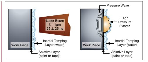
If the geometry allows expansion then forming such as wing panels for aircraft or corrective forming of structural parts can be achieved.
