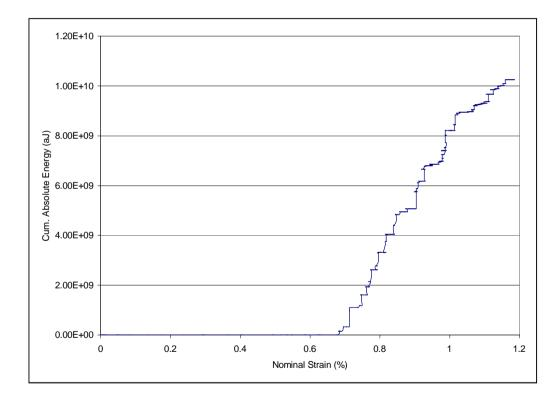
Plot of cumulative energy detected versus nominal strain on the coating surface for a typical HVOF WC-Co coating.
