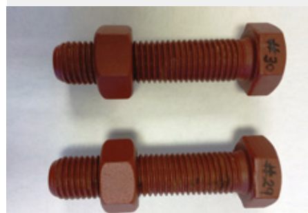
Coated Bolts after 1500 hrs Salt Spray Testing
