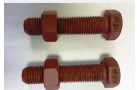
Coated Bolts after 1500 hrs Salt Spray Testing
