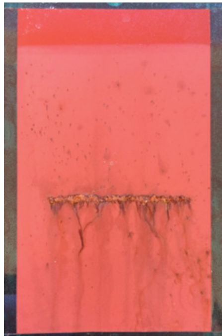
15 ISO20340 cycles current market leader - showing widespread blistering and a small level of creep from the scribe.
