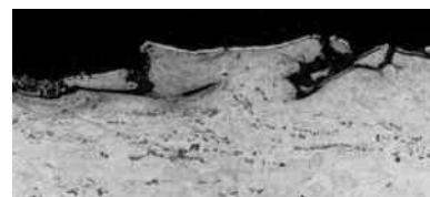
FIGURE 11-2A Damaged Surface from Broken Shot Media
