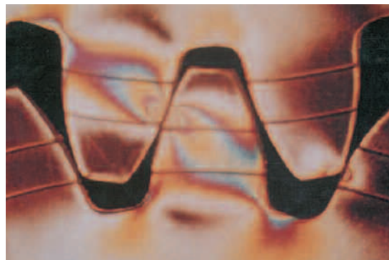
FIGURE 4-3 Polarized View of Applied Gear Stresses
