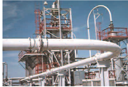
FIGURE 10-6 Manufacturing Plant Utilizing Directionally Textured Pipe
