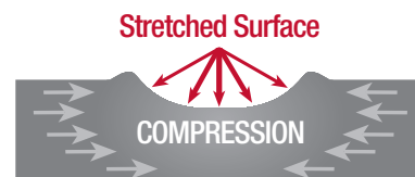
FIGURE 1-2 Compression Resists Fatigue Cracking
