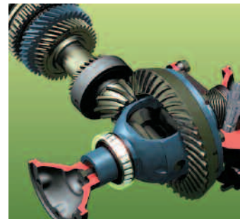
FIGURE 4-2 Ring and Pinion Gear Assembly
