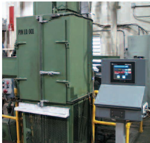
FIGURE 11-10A Computer Monitored Lance Shot Peening Machine for Processing Internal Bores
