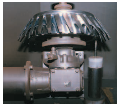
FIGURE 4-7 Lance Peening of Fan Disk
