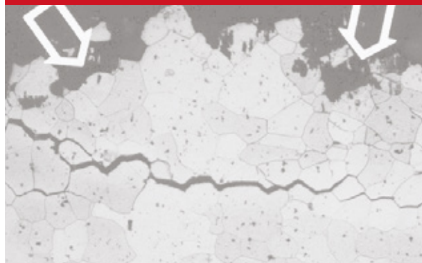
Fig. 8-3B Primary and Secondary Cracking from Intergranular Corrosion
