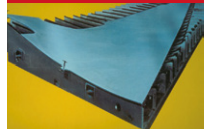
Fig. 10-2 Checking Fixture for Verifying Peen Forming of Wingskin
