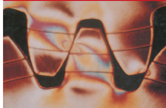
Fig. 4-3 Polarized View of Applied Gear Stresses
