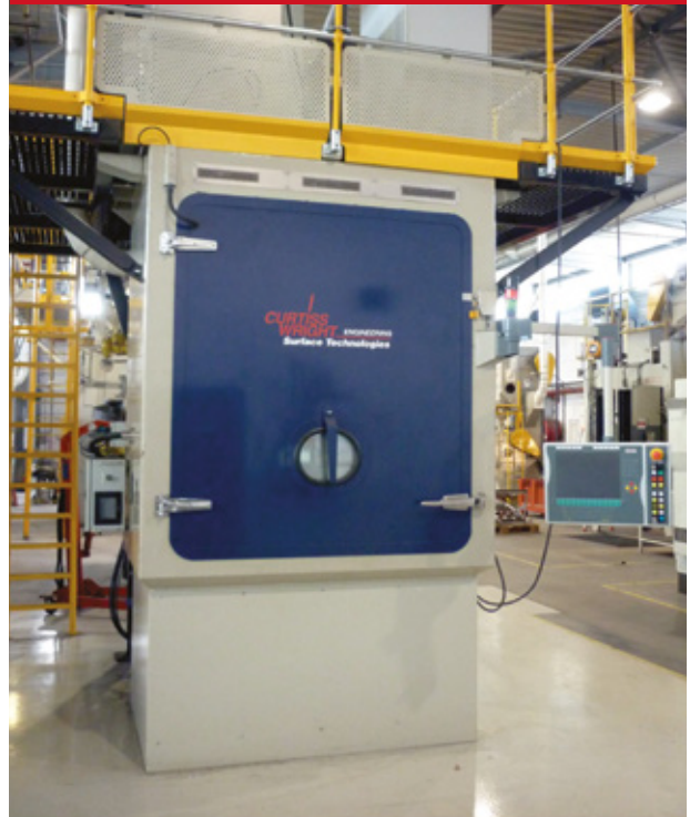
Fig. 11-10B Multi-Nozzle Computer Monitored Shot Peening Machine
