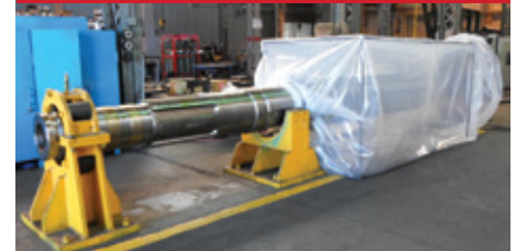
A work area that has been tented to protect facility and staff from flying media
