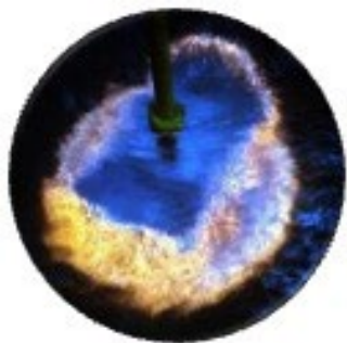
Fig.3. Component immersed in the electrolyte bath showing plasma discharge during the Keronite PEO process.
